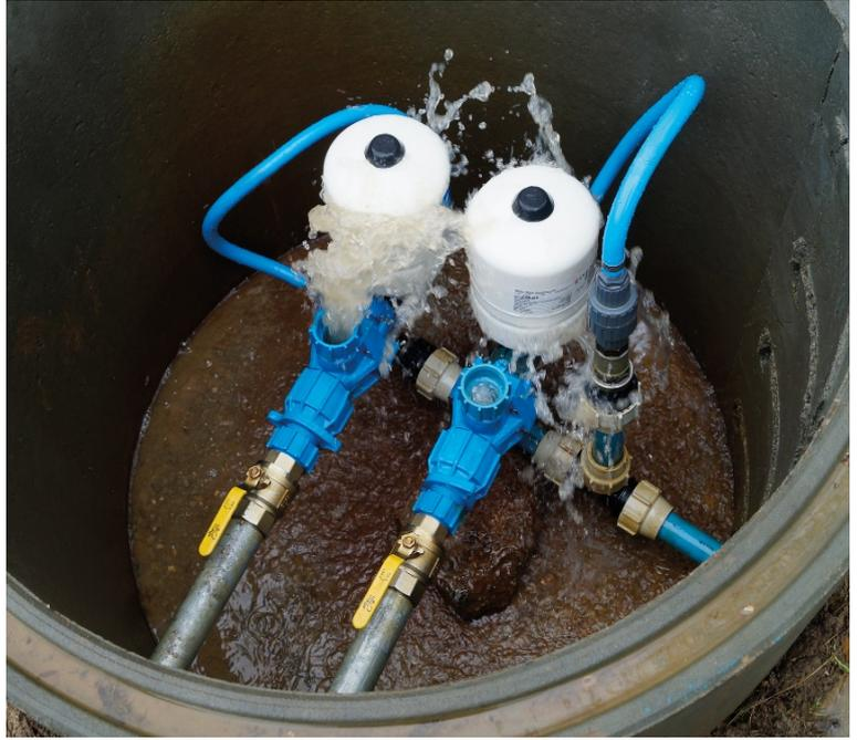
**The Papa Pump works without the use of any fuel or electricity – it just uses the natural power of flowing water.**
